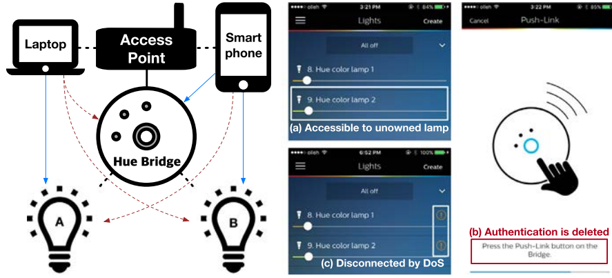
Fig. 1. An IoT network with commercial IoT devices - dash arrow and dotted arrow lines refer to valid and invalid accesses respectively.
