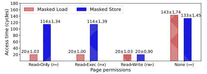
Fig. 5. A comparison of execution times according to page permissions. A masked load can distinguish two types of pages (r-/r-x and --), whereas a masked store can distinguish three types of pages (r-/r-x, rw-, and --).
